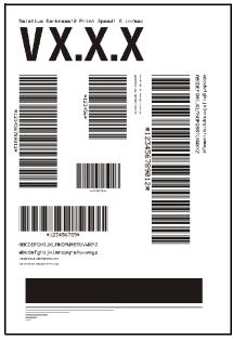
Inspect these labels and determine which one has the best darkness setting for your application. This value can be entered into the printer by setting the darkness during the configuration procedure.
